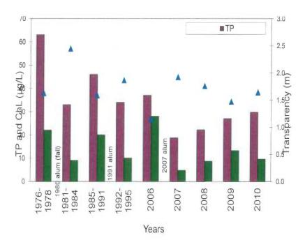
Figure 1. Mean whole-lake summer (June-September) TP, chl and Secchi transparency for groups of study years before and after three alum treatments in Long Lake, Kitsap. Pre 2006 data from Welch (1996). Data for 2006 serves as a partial reference for post-alum years 2007-2010.
